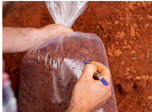
STEP 4. Store in plastic bags, tie with string, and identify the sample.
