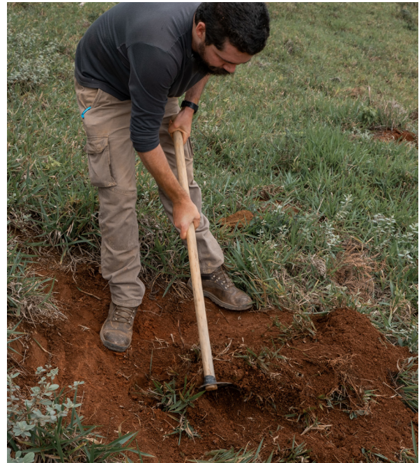
STEP 4. At the end of the collection, cover the open hole with the surface layer (A Horizon) that was removed in stage 1 and compact to avoid accidents and erosion.
