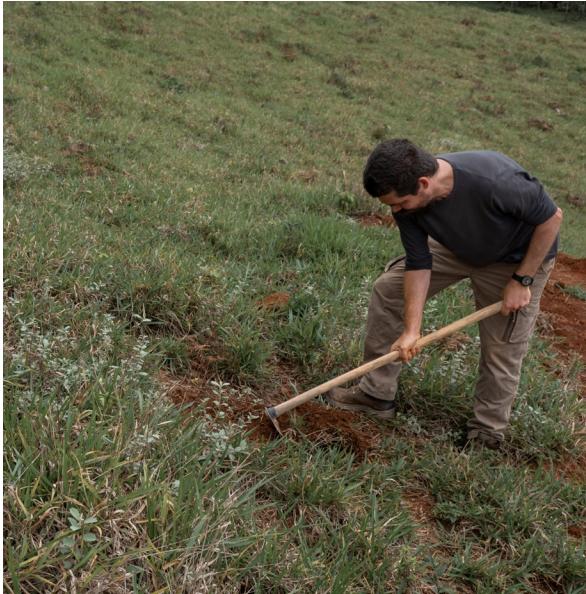
STEP 1. Remove the surface layer (A Horizon) with a hoe and reserve.
