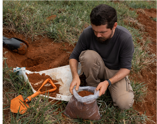
STEP 3. Store in plastic bags, tie with string, and identify the sample.
