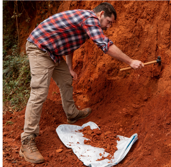
STEP 3. Underlay the base of the ravine with a plastic bag, dig with a hoe or rake and take samples evenly in different positions without opening holes to avoid damage to the ravine's structure and, thus, landslides and erosion. Take samples carefully to prevent contamination with materials of organic origin or other types of soil. Always clean the tools thoroughly with each collection.
