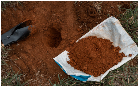
STEP 2. Dig with a hoe or digger to take samples carefully to avoid contamination with materials of organic origin or other types of soil. Always cover with a plastic bag and clean the tools thoroughly with each collection.
